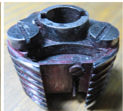
Both sides of a Universal cam showing the dater die and 7 Wavy line split obliterator in place
