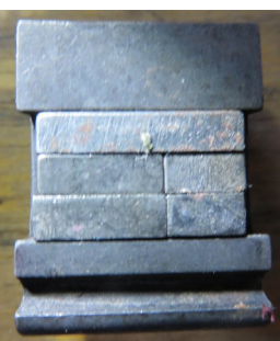
Back of dater die showing year, time and date slugs in place, and alongside. The groove locates with the spring affixed using one of the bolts
