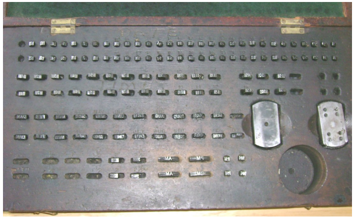
Krag hand operated machine and die box with two of each item needed for the two dater dies used to produce the distinctive continuous impression
