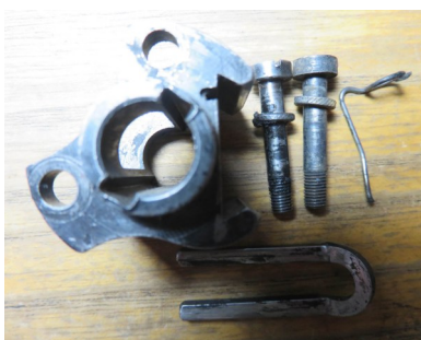
Cam, bolts for fitting obliterator, spring to hold dater die and central pin
