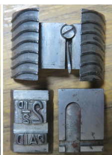
Wavy line obliterator and 2 1/2 PAID slug & back
