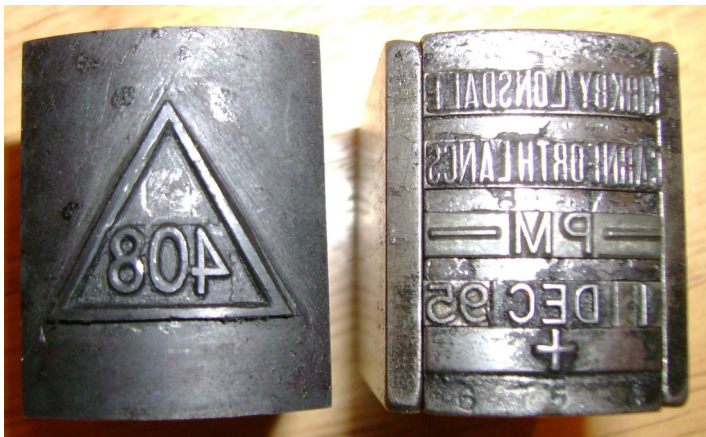
Krag printed matter and dater dies
