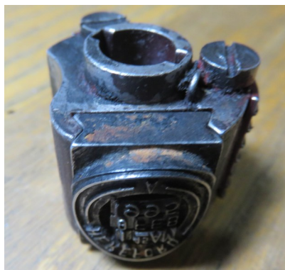
Both sides of a Universal cam showing the dater die and 7 Wavy line split obliterator in place
